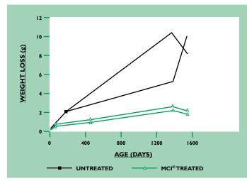
FIG. 4 MCI<sup>®</sup>-2020 long term test 1994-95 by General Building Research Corporation of Japan
